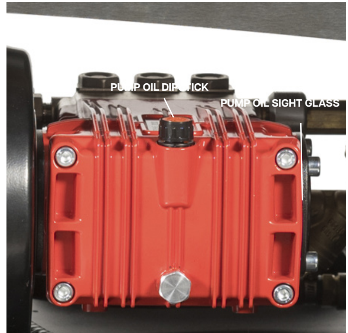
Figure.7 - Checking Pump Oil Level
