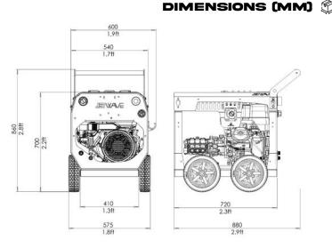
**HORNEL** 62 280-15 TECHNICAL DATA 0:00 CW4000-15PG2 **Product Code** Pressure / Flow Rate 4060PSI (280 BAR) / 15 L/PM (900 L/PH) / 4 GPM 60°C/140°F Max Water Inlet Temp Class (AS/NZS: 4223) A (4,200 Bar/Litres) Usage Frequency Professional: Daily Nozzle Size 04 Frame Structure CNC Modular galvanised sheet steel chassis plus satin powder coat finish and stainless steel cover
